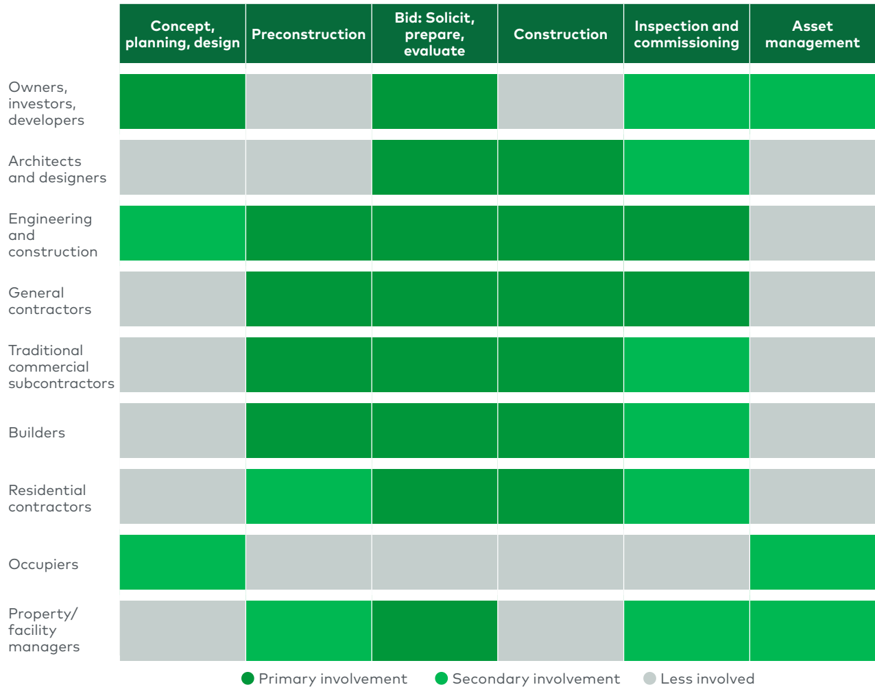
Figure 2 Stakeholder involvement at each stage of the building and construction management process
