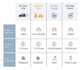
Note: Charge time based on a 40kWh battery size. DC High Power — Charge time is applicable when EVs are capable of this charging speed Source: L.E.K. and Tritium analysis
